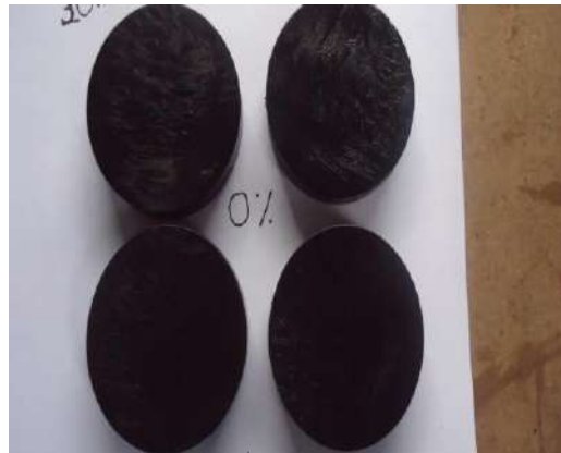
Fig 2.1.2 Thermal conductivity specimens
