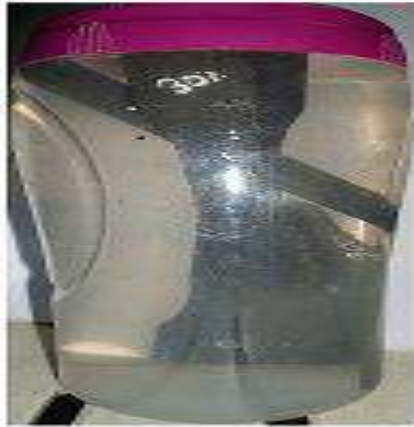
Fig 2.1.4 Water absorption specimens
